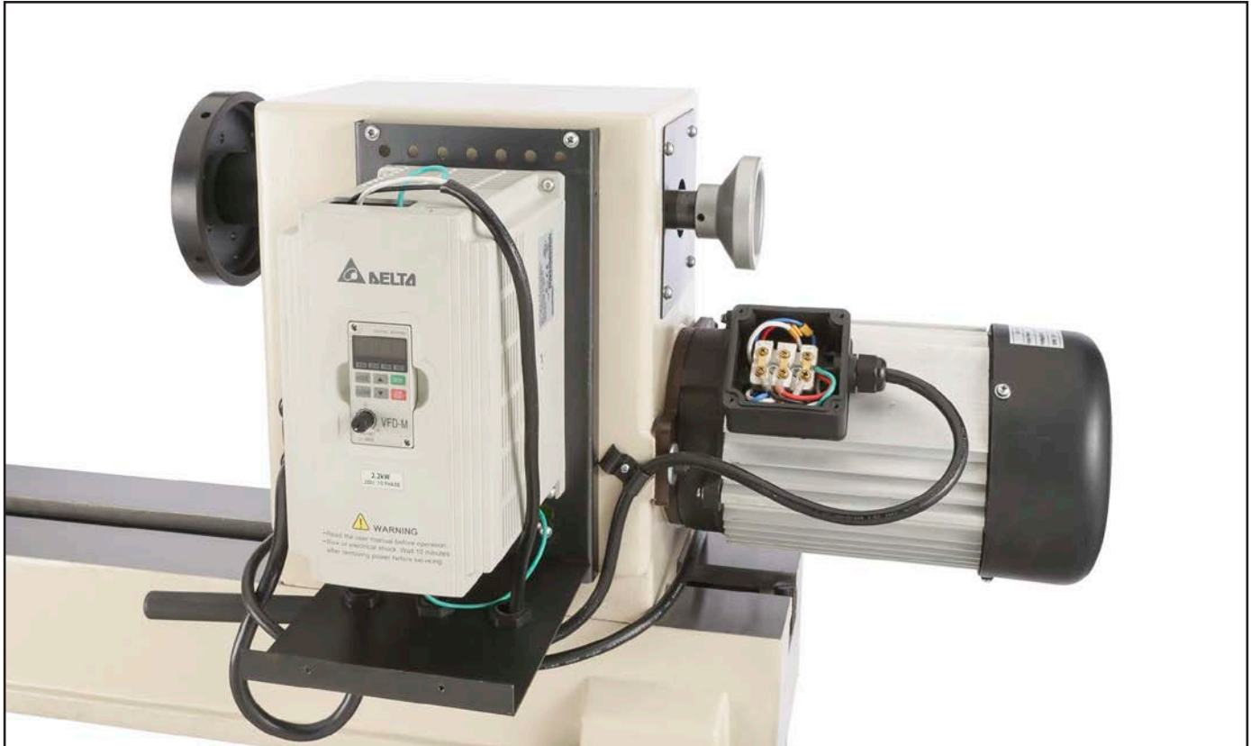
Figure 59. Inverter box and motor box locations.
